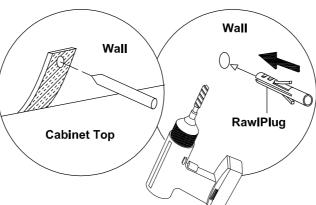
Drill a hole in the wall and insert the rawlplug.
