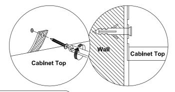
NOTE: Wall fixings are not supplied with this product as different wall materials require different types of fixing devices (such as Rawl plugs on brick work). You must use fixing devices suitable for the type of wall you intend to mount this product to.Please ensure that the head of any screw used has a diameter greater that the diameter of the mounting hole on the bracket and that the fixing is safe and secure before use.
