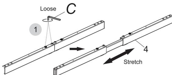
Loosen the screws (4) with wrench 4x4(C), then expand the supporting beam to required length.
