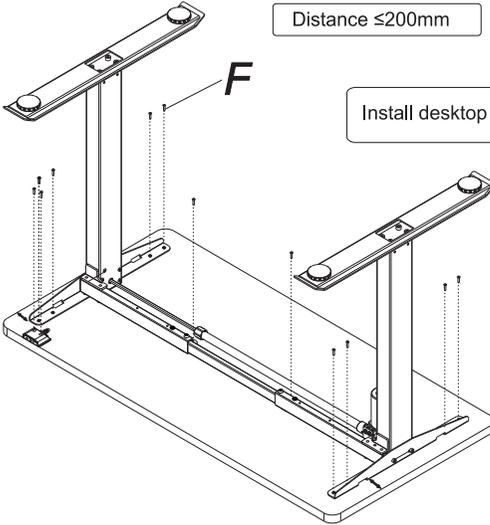
Install desktop with screw(F), use pistol drill to tighten.
