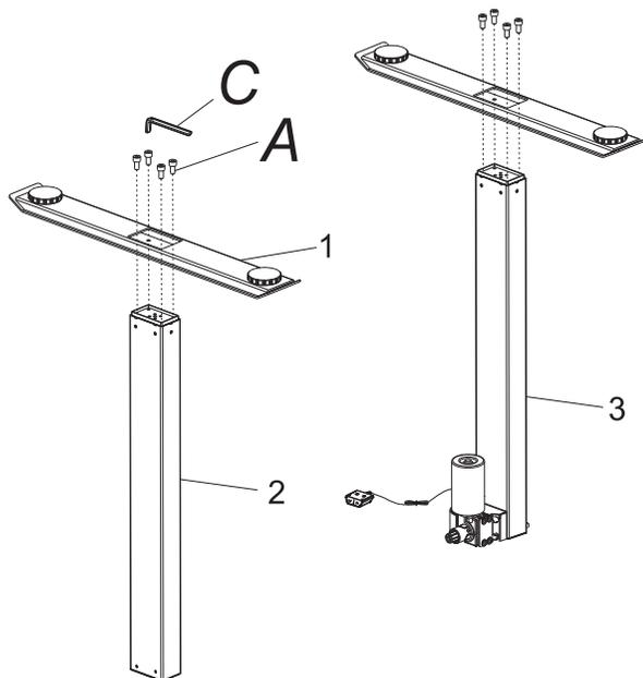
Install (1) & (2)(3) together, use 5\*5 wrench(C) to tighten the screws(A).
