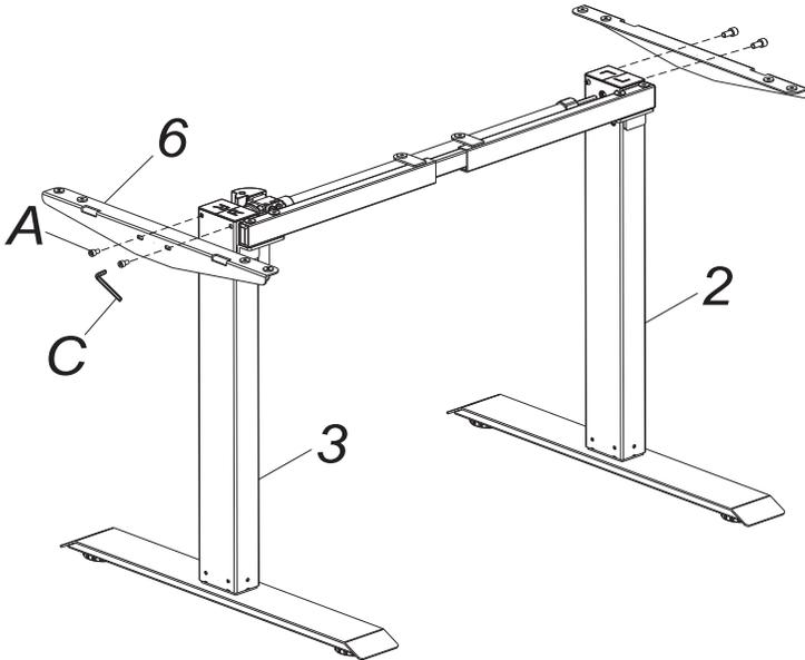
Install(6)&(2)(3), use 5\*5 wrench(C) to tighten the screws(A).
