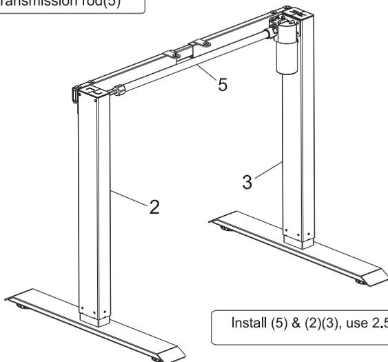
Install (5) & (2)(3), use 2.5\*2.5 wrench(D) to tighten(G).
