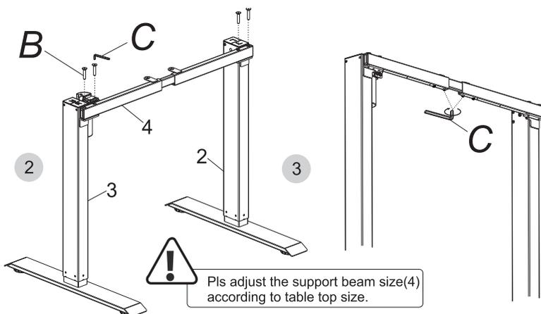
Install supporting beam on the column (2)(3), tighten screw (B) with wrench 5x5 (C)
