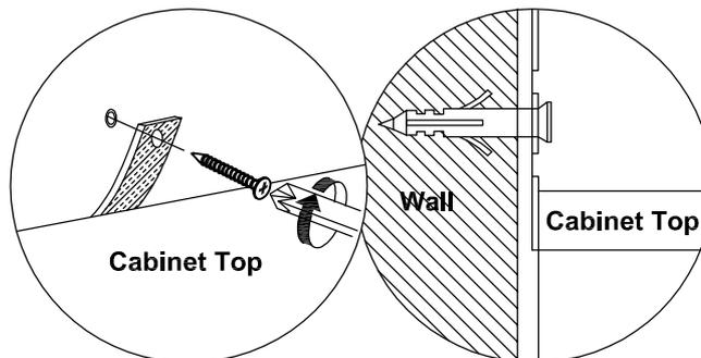
**NOTE :** Wall fixings are not supplied with this product as different wall materials require different types of fixing devices (such as Rawl plugs on brick work). You must use fixing devices suitable for the type of wall you intend to mount this product to. Please ensure that the head of any screw used has a diameter greater than the diameter of the mounting hole on the bracket and that the fixing is safe and secure before use.
